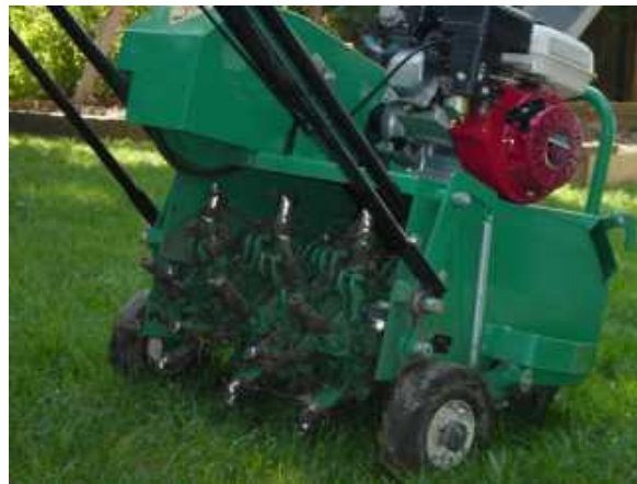
A core aerator's tines pull plugs of soil from the lawn.
